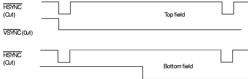
Figure 9-16 \overline{VSYNC} and \overline{HSYNC} Out
